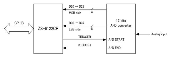
It does A/D START with TRIGGER and generate SRQ with A/D END or A/D BUSY termination. However, in case of high-speed operation where A/D operates in several tens  $\mu$ s, there is a case that a method of reading data immediately after A/D START may be used without using SRQ.
