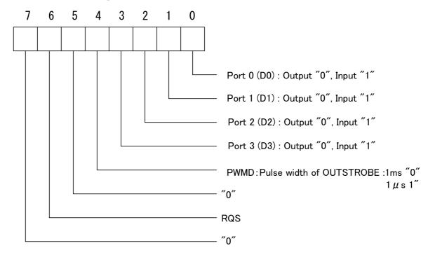
For RQS, an interrupt is generated by the REQUEST signal of pin 22 of the data connector, SRQ switch of the front panel is ON, and this bit becomes "1".
